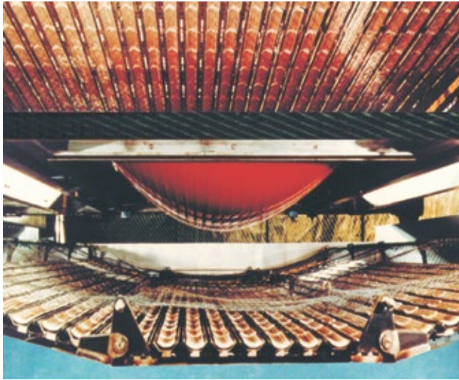
Figure 7: Thermoforming plant for boat hulls
